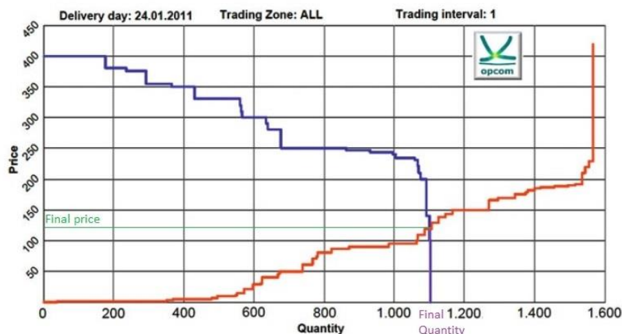
Figure 12: Example of the clearing of an aggregated demand (blue) and supply curve (red) for one hour of the DAM in Romania on 24/01/2011 (Pérez-Arriaga, 2013).
